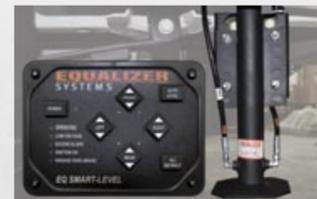
**Automatic, 4-Point Hydraulic Leveling Jacks with Bluetooth Smart Phone App Control**
